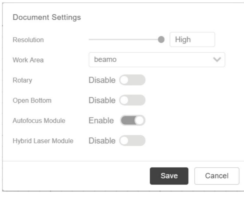
Note: Only when beamo is installed with the autofocus add-on can this function be enabled.
